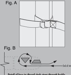
Detail of how to thread cinch strap through buckle.
